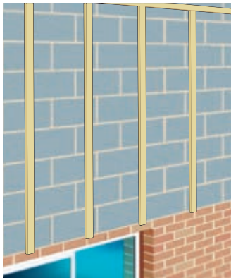
Fix perimeter frame and intermediate vertical battens to wall.
