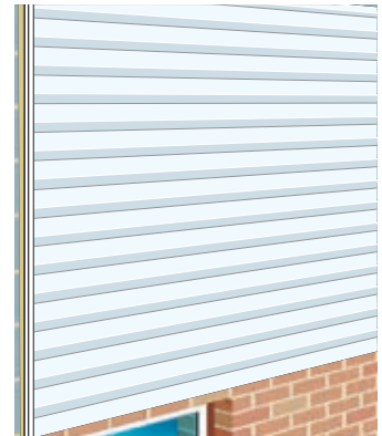
Fit remaining planks and engage male part of two part trims.
